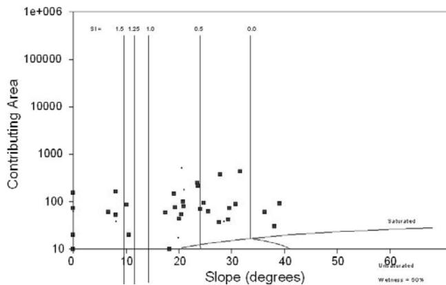
Figure 7. Slope (degrees) - Area (m<sup>2</sup>) Plot of Fraser Hill Catchmen Based on the SA plot, 73.5% of the landslide occurred on slope of more than 10 degrees. However there were also landslide occurred in flat areas especially those located in the Fraser Hill town which caused by modification of road. Detailed interpretations of the SA Plot were provided as the statistical summary in Table 6 and Table 7 for 2 and 4 meters soil depth respectively.
