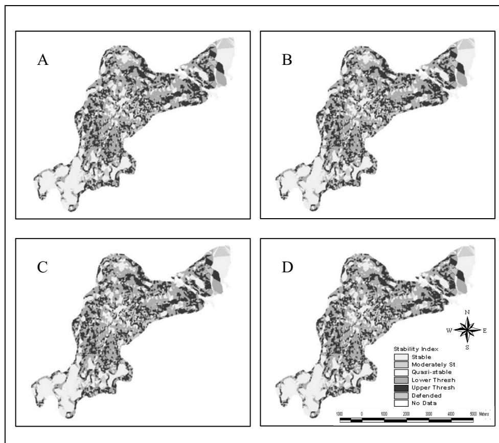
Figure 5. Stability index grid map based on four precipitation events. A, B, C and D represent SI map using 10mm, 30mm, 70mm and 110mm of precipitation respectively. The soil depth is 2 meters.
