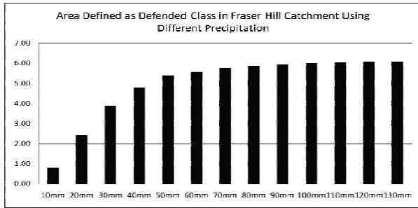
Figure 4. Percentage of Defended area according to different precipitation event for 2 meter of soil depth
