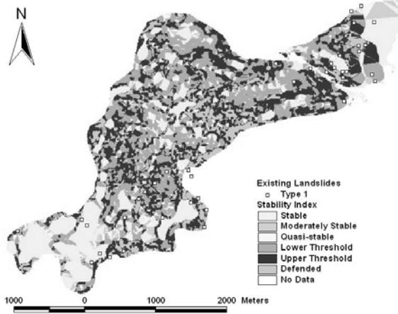
Figure 6. SI map for soil depth equal to 4 meters and rainfall is 110mm
