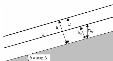
Figure 3. Infinite Slope Stability Model Schematic (Pack *et al.*, 1998)
