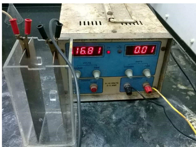
Figure 1. Experimental setup for electrocoagulation
