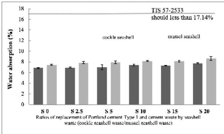
Figure 6. Water absorption of concrete bricks with replacement of Portland cement Type 1 and cement waste by seashell waste (cockle seashell waste/mussel seashell waste)
