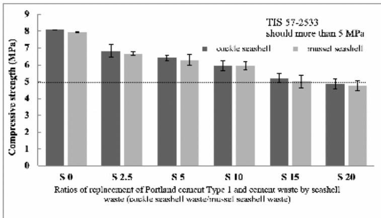
Figure 7. Compressive strength of concrete bricks with replacement of Portland cement Type 1 and cement waste by seashell waste (cockle seashell waste/mussel seashell waste)
