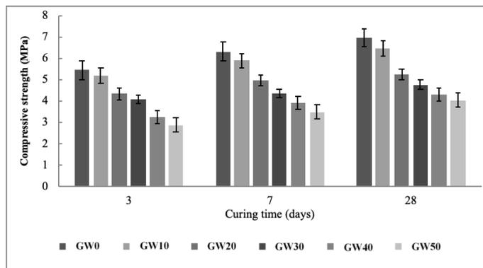
Figure 11. Compressive strength of concrete bricks (ratio obtained from 3.2.3 using mussel seashell waste) with replacement of sand by glass waste
