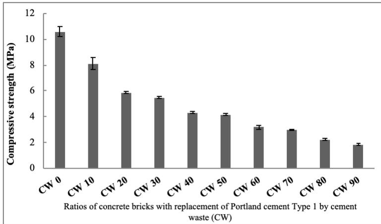
Figure 5. Compressive strength of concrete bricks with replacement of Portland cement Type 1 by cement
