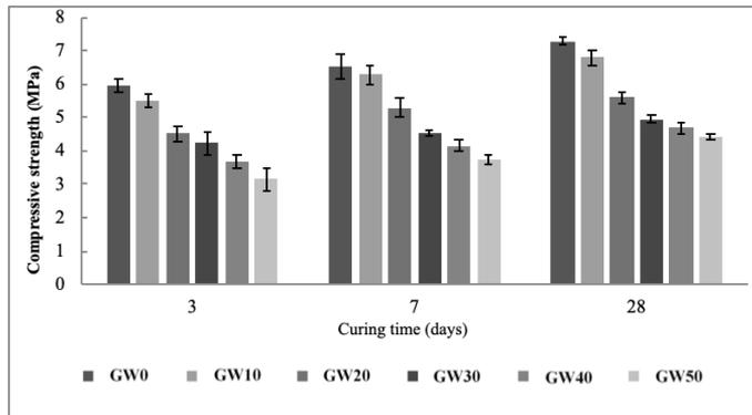
Figure 10. Compressive strength of concrete bricks with (ratio obtained from 3.2.3 using cockle seashell waste) replacement of sand by glass waste
