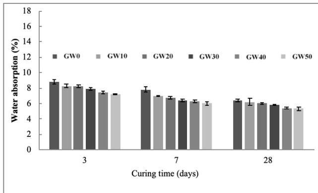
**Figure 8.** Water absorption of concrete bricks (ratio obtained from 3.2.3 using cockle seashell waste) with replacement of sand by glass waste
