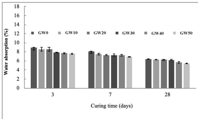
**Figure 9.** Water absorption of concrete bricks (ratio obtained from 3.2.3 using mussel seashell waste) with replacement of sand by glass waste
