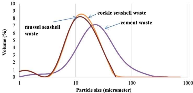
Figure 3. Particle size of raw materials
