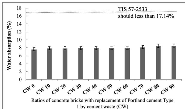
**Figure 4.** Water absorption of concrete bricks with replacement of Portland cement Type 1 by cement waste
