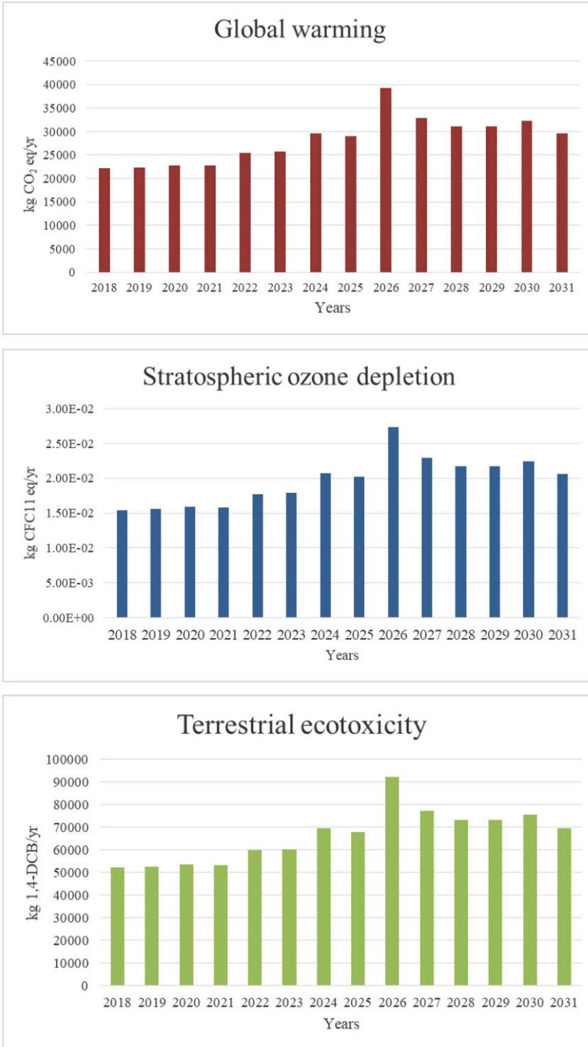
**Figure 4.** The prediction of environmental impacts; i.e., global warming, stratospheric ozone depletion, and terrestrial ecotoxicity, from landfill method for rigid polyurethane foam waste
