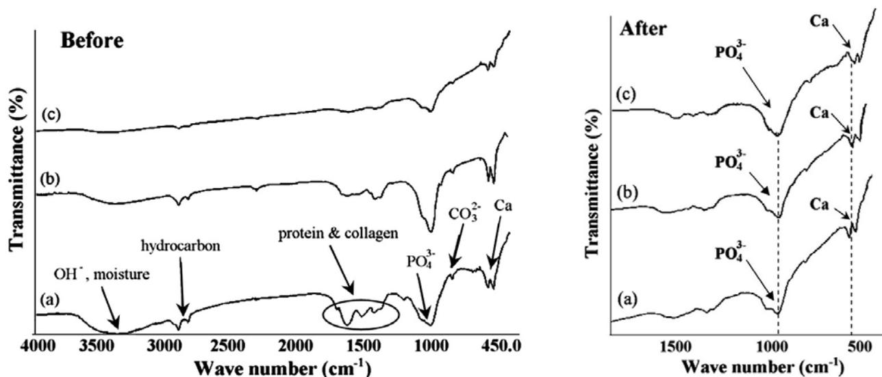
Figure 2. FTIR spectra of bone (a) bone char (b) and activated bone char (c) before and after sorption of lead
