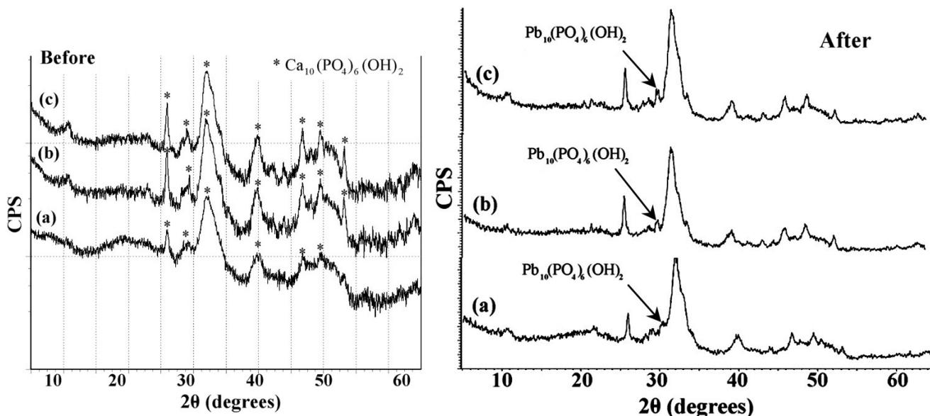
Figure 3. X-ray diffraction patterns of bone (a) bone char (b) and activated bone char (c) before and after sorption of lead
