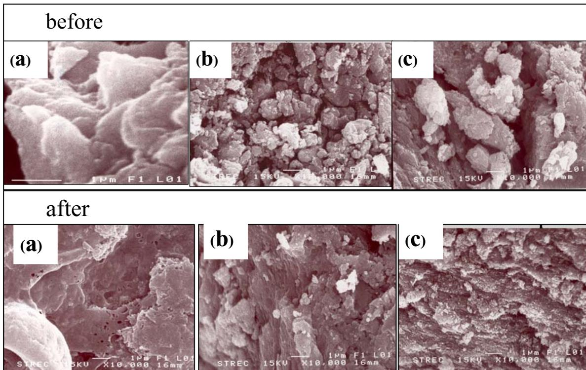
Figure 1. Electron micrographs of the three sorbents: bone (a), bone char (b) and activated bone char (c) from SMEs, ×10,000 (before and after sorption)
