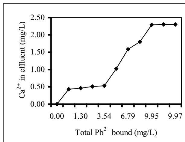
Figure 4. Relation of total lead ion bound and amounts of  $Ca^{2+}$  release. Conditions: initial lead ion concentration 10 mg/L; pH  $5 \pm 0.1$ ; volume 50 ml; bone char weight 0.005 g.
