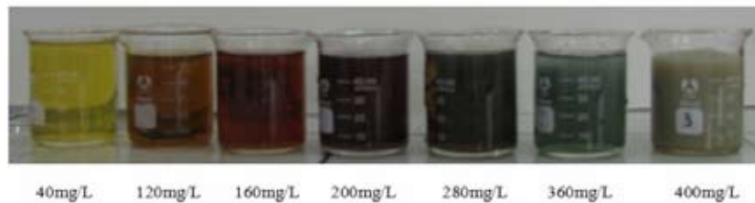
Figure 5. The solution color changing vs silver concentration
